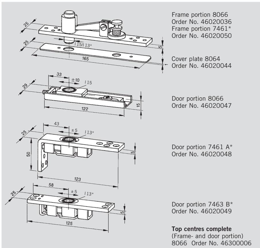
\* For door portions 7461 A and 7463 B, use frame portion 7461 with 13 mm dia. pin.
