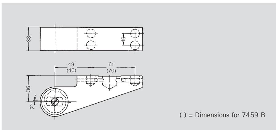
**Drill jig for aluminium hinges**
